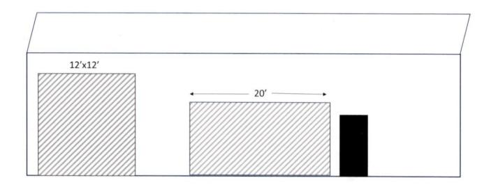
Add additional garage door. This garage door should line up with the existing garage door farthest to the right from the front view.
